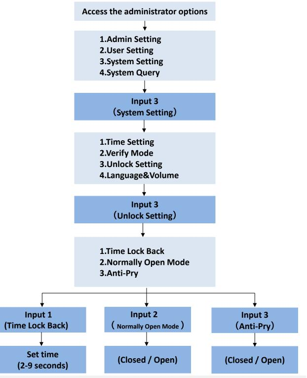
Note: Activate the "Normally Open Mode "mode with caution! The "Time Lock Back "refers to the duration before the deadbolt re-engages after unlocking.
