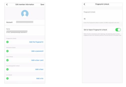
Attention: When using a hijack alarm user to unlock the door, the lock will open normally without sounding an alarm. However, an alarm message will be pushed to the App. . The alarm information will not be uploaded to the cloud if the door lock is not connected to the network when the door is unlocked.
